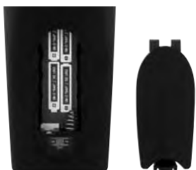
Figure 18 – Remote Battery Compartment
